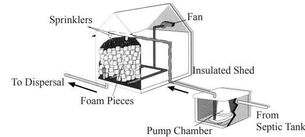
**Synthetic media** such as foam or textile filters are used as surfaces for sprayed pretreated (solids are settled out) wastewater where bacteria use the nutrients in wastewater as a food source. The foam or textile filter may be followed by a polishing sand filter and shallow infiltration trenches to provide the final treatment and dispersal.
