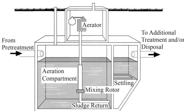
An **aerobic treatment unit** generally is preceded by a septic tank to collect and pretreat the solids with anaerobic (without oxygen) digestion. This reduces the amount of solids passing into the aerobic treatment where bacteria that need oxygen (aerobic) digest the waste. Some aerobic systems have solids settle in a separate compartment which requires periodic pumping. Further treatment and/or disinfection is needed before final release into the environment.
