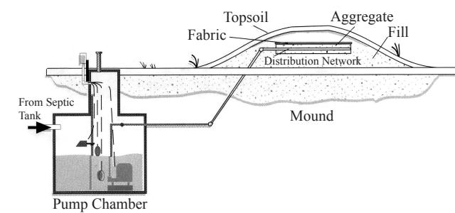
A **pressure mound system** provides a soil absorption site that is raised above the natural soil surface. It overcomes the problems of slowly permeable soils, shallow permeable soils over clay or permeable soils with high water tables. Wastewater from the septic tank is pumped to the mound and dosed on suitable fill material.
